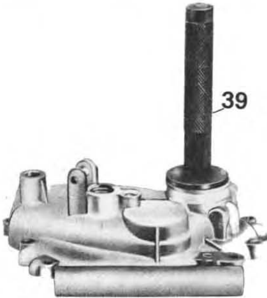
Installing the layshaft seal
