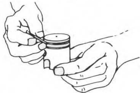
Decarbonizing the ring grooves
