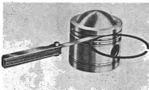
Checking ring-to-piston-side clearance
