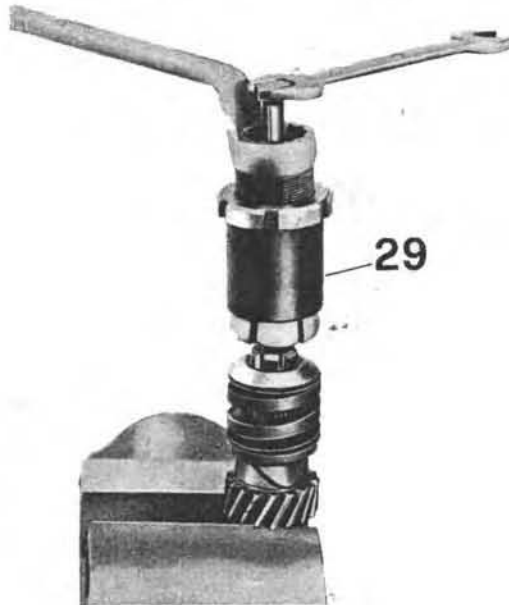
Removing the clutch shaft inner bearing race
