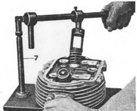
Removing the valves with the special tool
