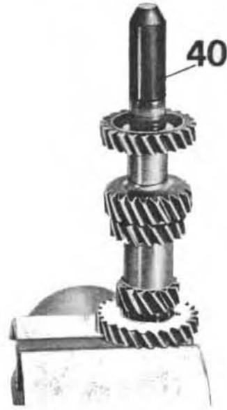
Installing the mainshaft bearing inner race
